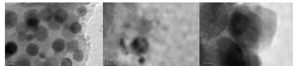
SEM electron micrograph of effective components of aluminum hydroxide in adsorbent channels
