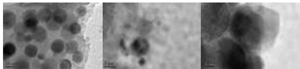
SEM electron micrograph of effective components of aluminum hydroxide in adsorbent channels
